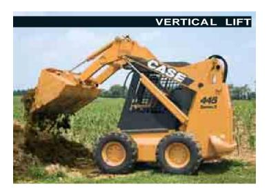
On 435, 445 series 3 the kinematics is of the vertical type. This means that the arm is articulated at its base by a heavy lift and reach linkage which makes loading/unloading in elevation easier. As for the radial lift units, the arm is in contact with the chassis in its low position giving these models good digging abilities as well.
