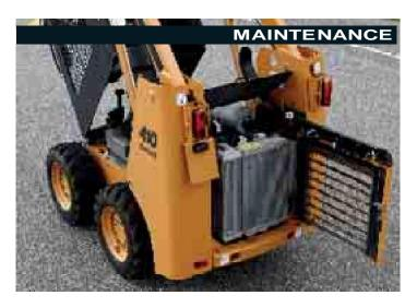
Regular service items can be easily accessed through a lift up panel on top of the engine cover and af ull swing-out door to the rear of the machine. For more in-depth maintenance the entire cab structure can easily be tilted forward, in less than a minute to provide unparalleled access to the can inner components of the machine.
