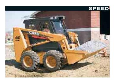
Productivity on 420, 430, 440 series 3 is vastly improved by blazing two-speed travel of 17 to 18 km/h. 410 with one speed only reaches 10 km/h.
